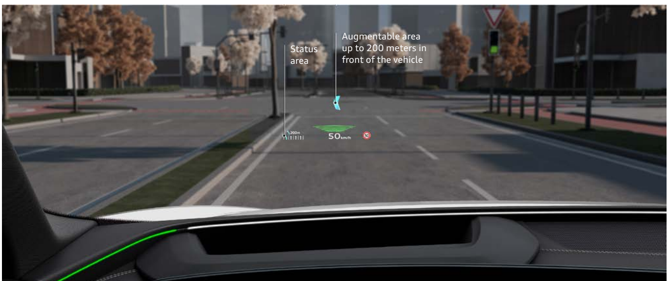
AR HUD 6 in the Audi Q6 e-tron: The displays can be understood quickly without distracting the driver.
