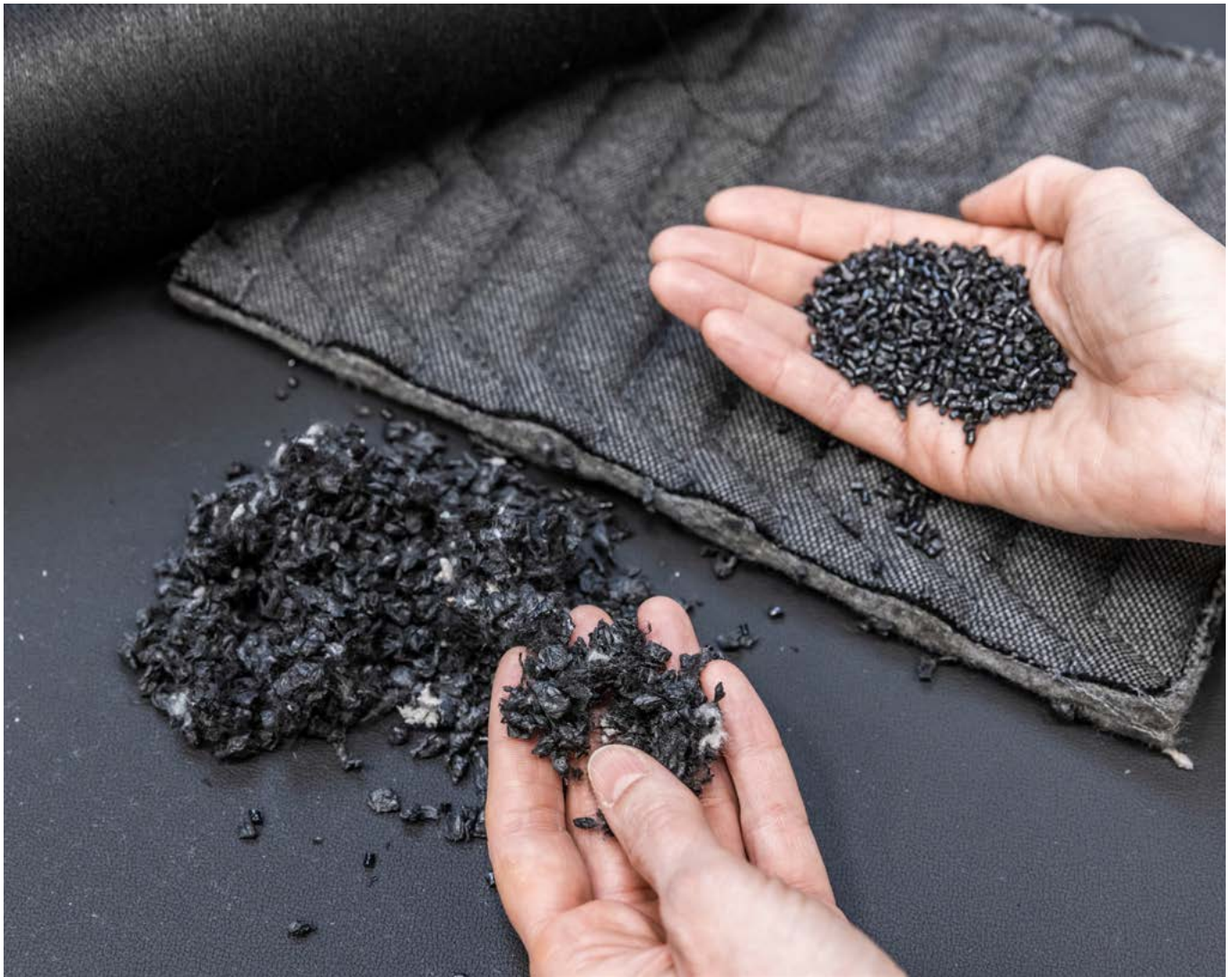
Recycled monomaterial seat covers can be used to make new yarn.
